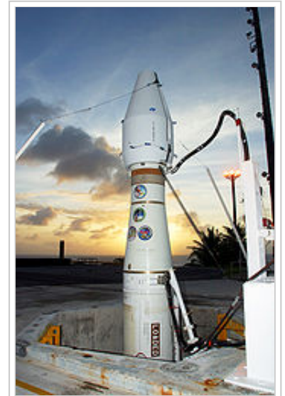
Ground-based Midcourse Defense (GMD) interceptor in launch silo at Vandenberg
