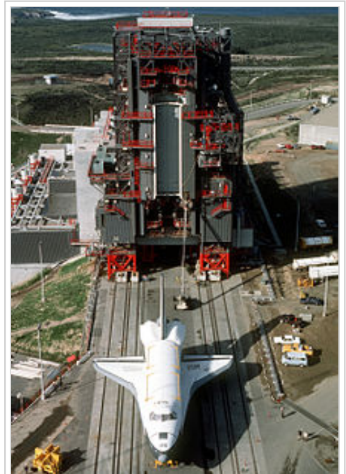
1985 photo of Space Shuttle Enterprise (OV-101) moving toward the shuttle assembly building at Vandenberg AFB Space Launch Complex 6 aboard its specially designed Cometto 76-wheel transporter. In the background are the payload changeout room and the payload preparation room.
