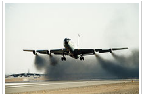
A KC-135A taking off with water injection to its J-57 engines
