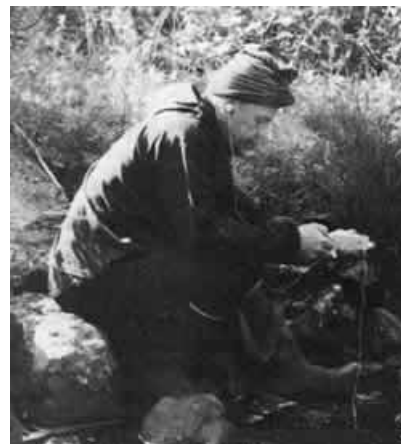
Erik Eriksson using a portable conductivity meter during a study of acidification and fish life in the mountains of Jämtland. When the balance was correct, the signal in his ear stopped.
