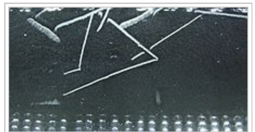
Radon220 decay in a cloud chamber
