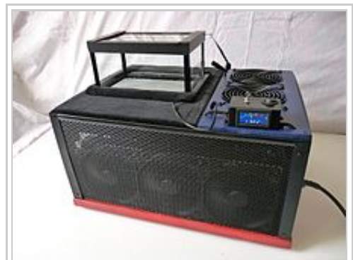
Example of watercooled thermoelectric cloud chamber
