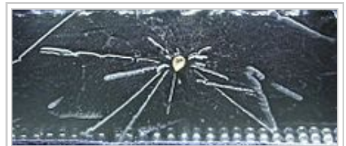
Radioactivity of a Thorite mineral seen in a cloud chamber
