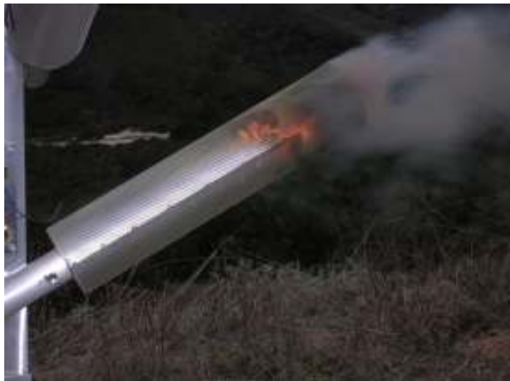
Figure 5.8 Flare burning inside a spark arrestor
