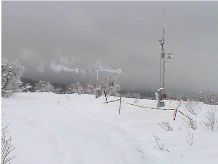
Figure 4. The central propane dispenser and tower at the High Altitude Seeding (HAS) location with the view toward the south-southeast where the Wasatch Plateau top is in cloud. The propane controller and data logger are at the base of the tower.
