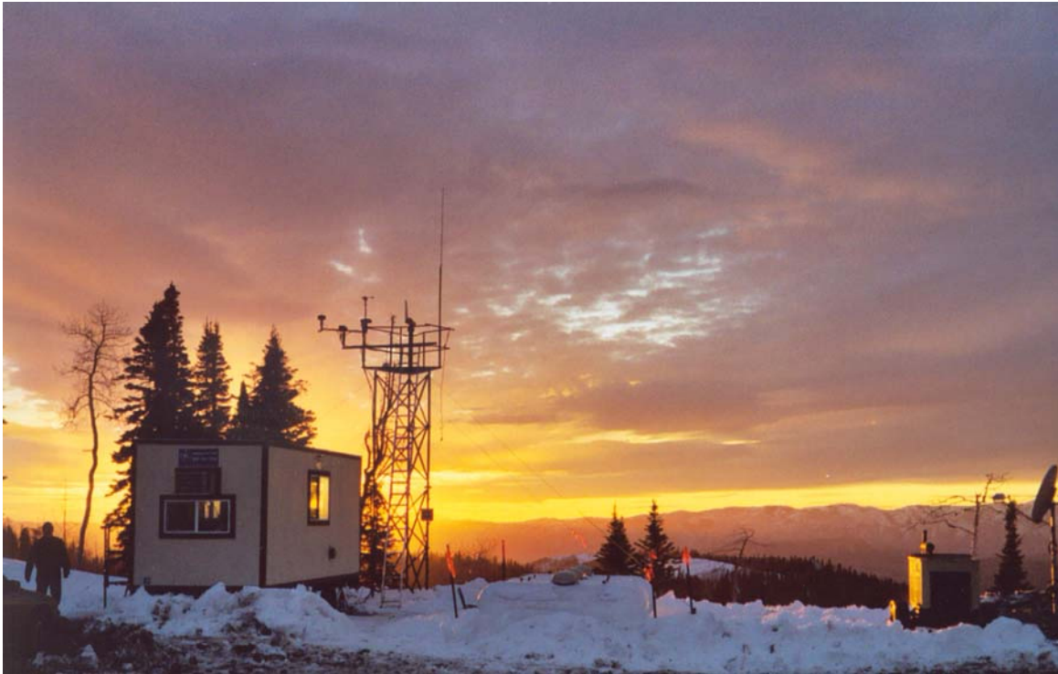
Figure 2. The TAR instrumented target facilities in early winter looking toward the west-southwest. The power generator and satellite dish for Internet connection are on the far right. The instrumentation platform was immediately west of the heated trailer which housed computers, electronics and other equipment.
