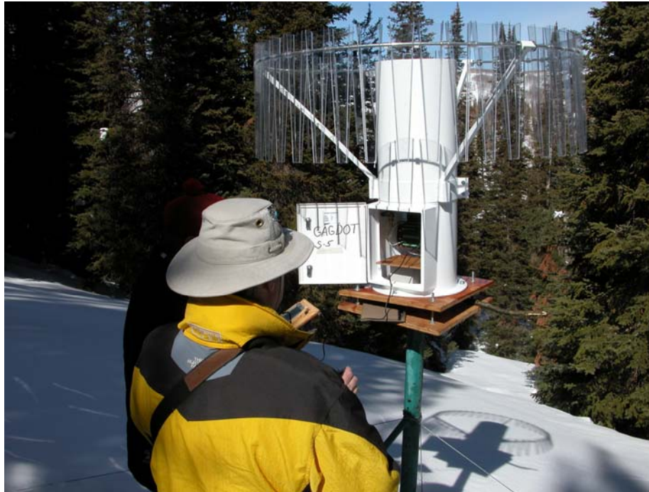
Figure 3. The high resolution precipitation gauge at the north control site with the view toward the north. In this picture, gauge data logger data are being downloaded to a portable Palm Pilot device. The 12-inch diameter gauge orifice is surrounded by an Alter-type wind shield made of clear Lexan plastic.
