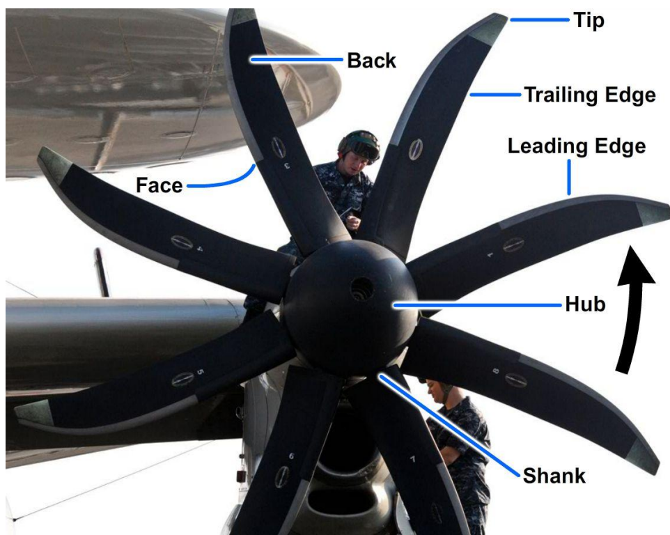
Figure 8-10 — NP 2000 (8) propeller blades.
