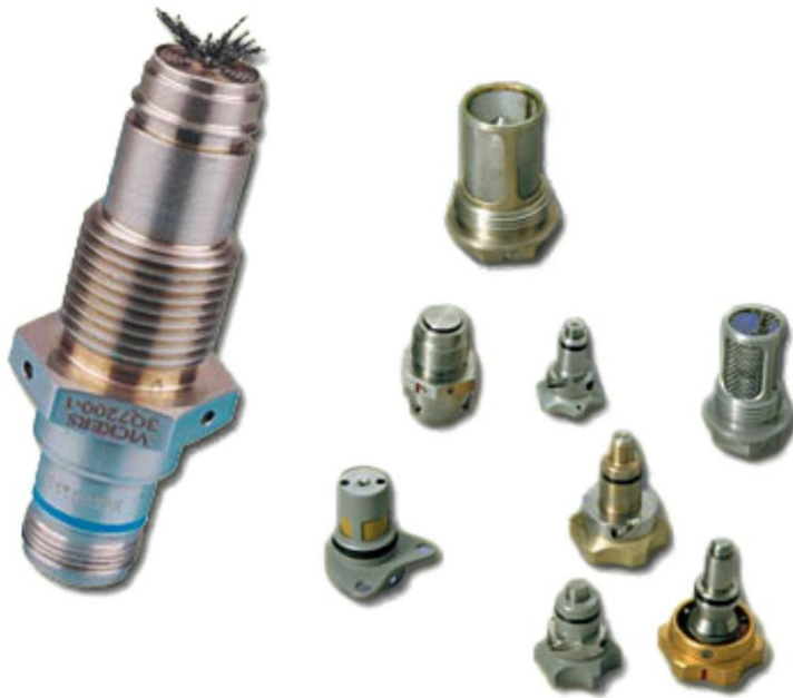
Figure 5-16 — Types of magnetic drain plugs with contamination.
