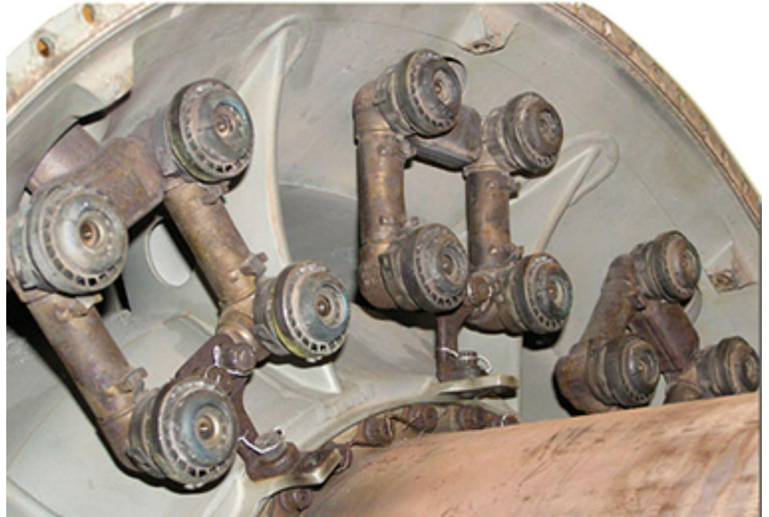
Figure 4-20 — Duplex fuel nozzle.
