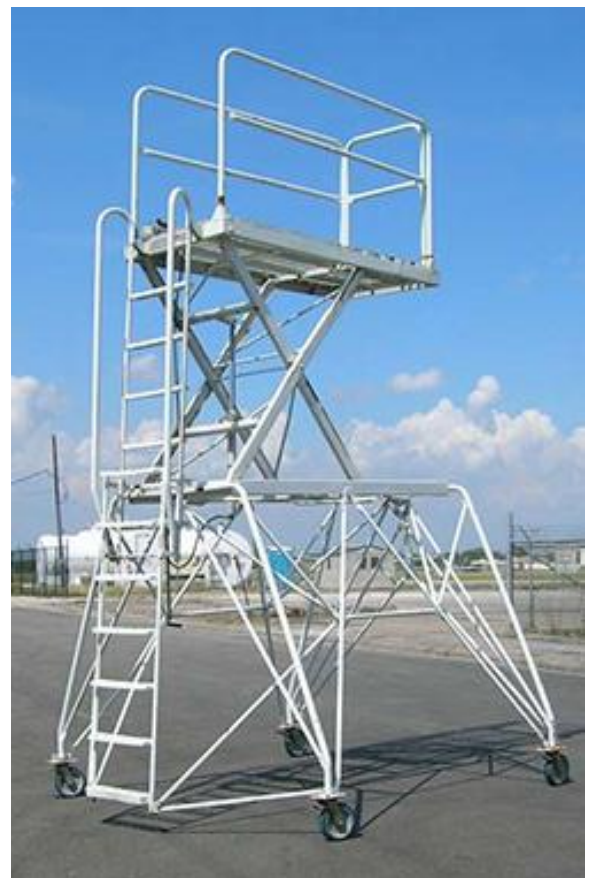
Figure 3-10 — B-5A Maintenance Platform.
