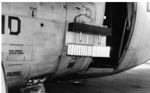
Fig. 6 – Photo showing pyrotechnic cloud seeding flare dispenser mounted on C-130
