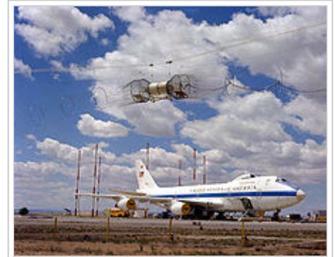
A right front view of a USAF Boeing E-4 advanced airborne command post (AABNCP) on the electromagnetic pulse (EMP) simulator (HAGII-C) for testing.
