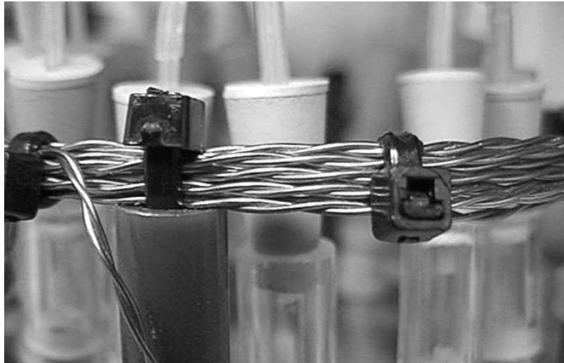
Fig. 2. Detailed view of the coil with the double filament wire. In active condition, current flow is in one filament only, while in inactive condition, current flows through both filaments in opposite directions, so that no magnetic field is produced.
