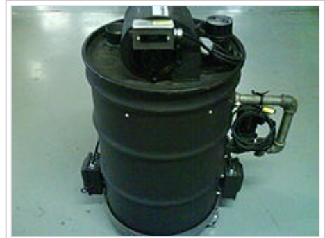
Generic Dry Ice machine made from a 3G. drum.
