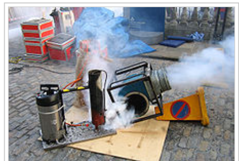
A heavy duty smoke machine feeding smoke into a blower to generate fog effects for open air location filming.
