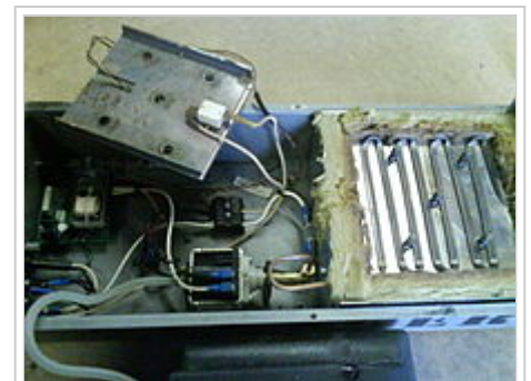
Interior view of a fog machine, showing the pump and heat exchanger.
