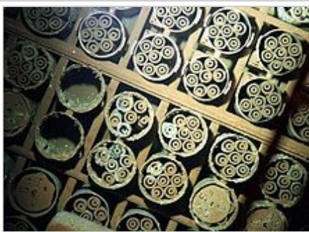
Spent nuclear fuel stored underwater and uncapped in Hanford's K-East Basin
